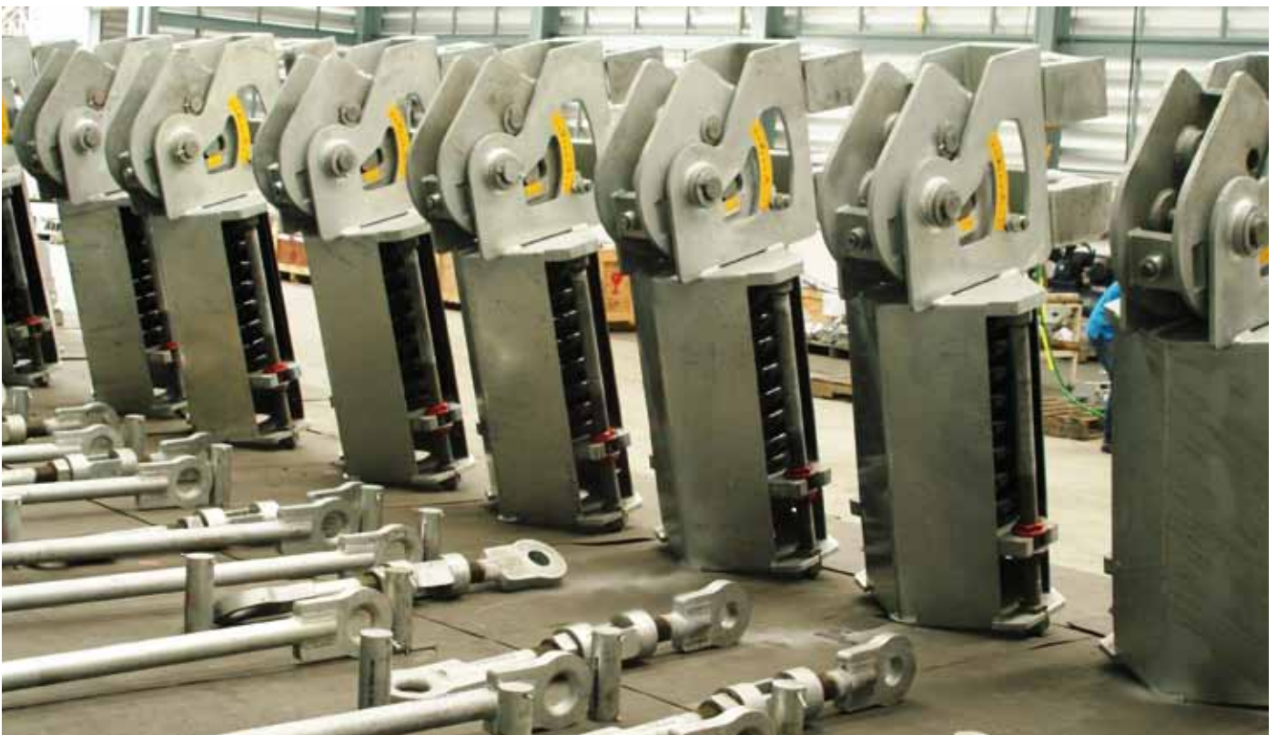
Constant effort pipe supports supplied to the Sadara petrochemical project in Saudi Arabia.
