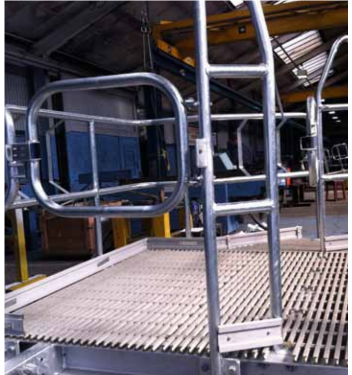
Steel platform with a GRP pultruded flooring section, ready for despatch and installation on an oil and gas rig.
